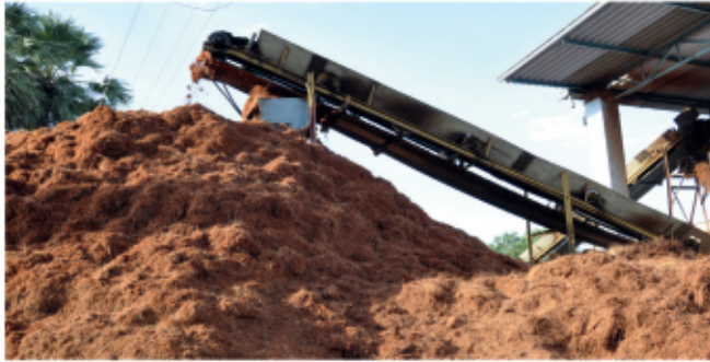
Milling systems separate coir pith and fibre.
